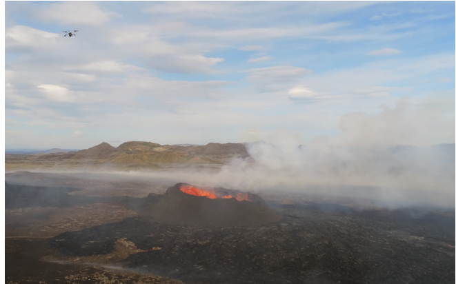
Fig. 1: A UNM VolCAN Dragonfly drone flying into the plume of the actively erupting Litli-Hrtur volcano in Iceland. This expedition involved measuring CO 2 concentrations across multiple transects of the plume to build a plume model and estimate the flux of the eruption.
